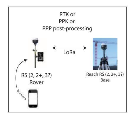
The rover can be replaced with an RS receiver and LoRa can be used for RTK (without NTRIP).
